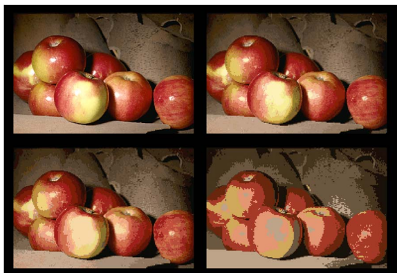
Fig. 2. (Color online) An example of a single difference scaling trial. On each trial, the observer sees two pairs of images and judges which pair (upper or lower) has the greater perceived difference. The upper pair corresponds to images compressed by factors of 6 (left) and 15 (right), the lower pair to images compressed by factors of 18 (left) and 27 (right).
